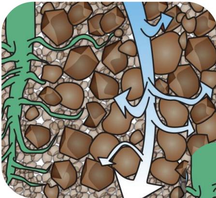
Without proper soil structure or the use of a surfactant, water flow is concentrated within the macropores.
